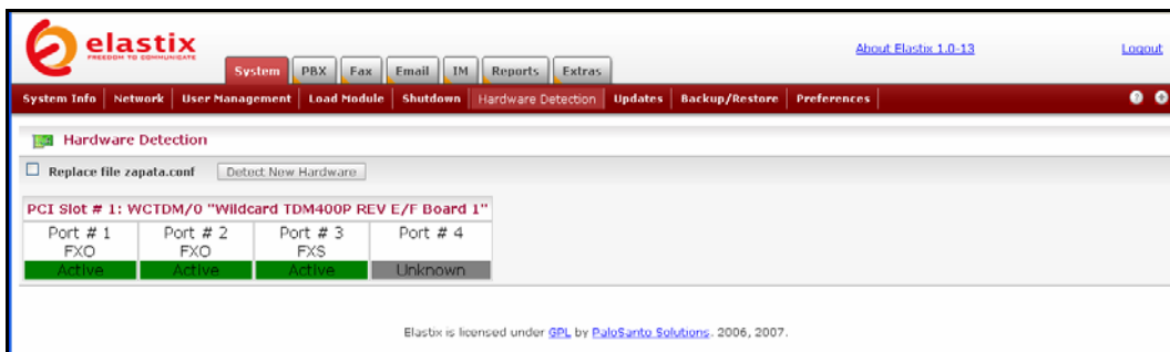
A400P with 2 FXO and 1 FXS modules installed
